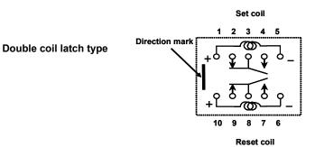
Double coil latch type (Reset position)
