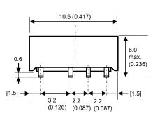
Tolerance of lead pitch is  $\pm 0.15 mm$  (0.006inch) Other tolerances  $\pm 0.3 mm$  (0.012inch) Coplanarity of terminals is 0.1mm Max.
